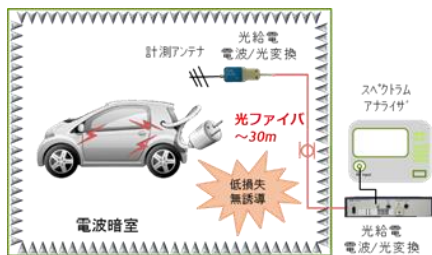
Illustration 1: The system testing for electrical noise
